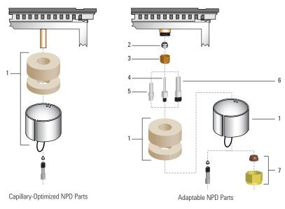
Nitrogen Phosphorus Detector (NPD) assembly (bottom)
